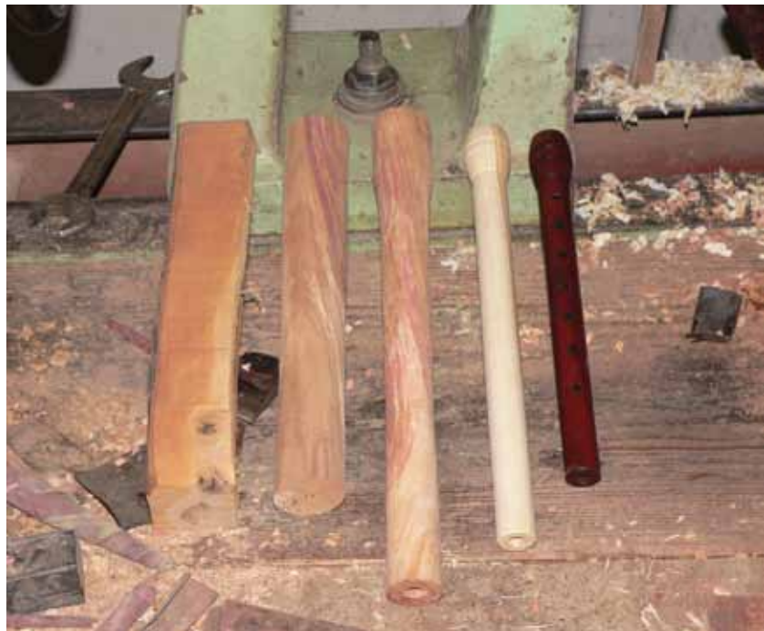
Figure 5. The bodies of five instruments at various stages of construction, displayed in the workshop of Ahmet Er, Istanbul. (photo courtesy Yalcın Savas)
